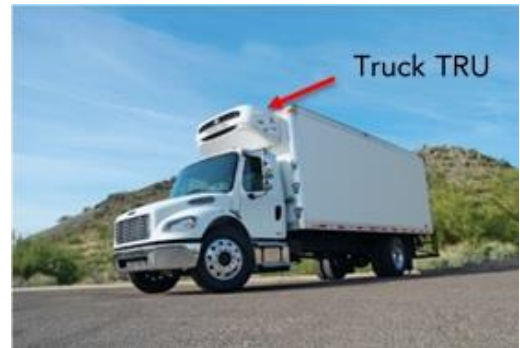
FIGURE 47. TRANSPORT REFRIGERATION UNIT MOUNTED ON TRUCK
