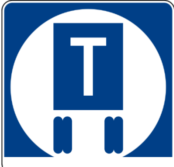
FIGURE 10: STAA TERMINAL ACCESS SIGN
