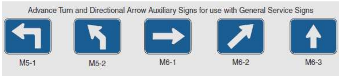
Figure 10: Advance Turn and Directional Arrow Auxiliary Signs
